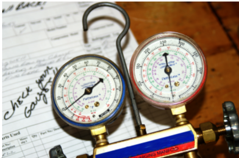
Calibration errors have become very common with the use of low loss fittings. This set pulled right from service may have caused numerous problems.
